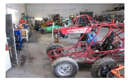
After suspension, add a motor. These are air and oil-cooled V-twin engines that are light but powerful. Finally, the disc brakes, bucket seats, racing-style harnesses, and steering are installed, and it's ready for fun! We typically build 1- and 2-seat buggies but have 4, 5, and even 6-seat buggies for families or larger groups. Our fleet represents the diversity of the venues at which we facilitate adventures!
